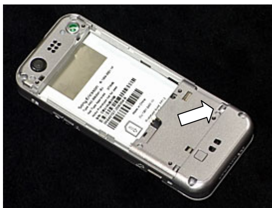
Location of the Liquid Intrusion Indicator.
