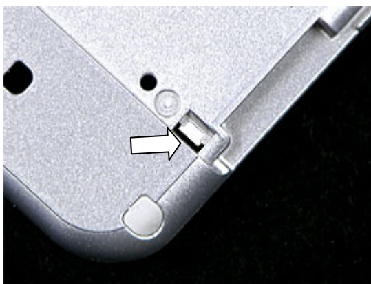
Location of the Liquid Intrusion Indicator.
